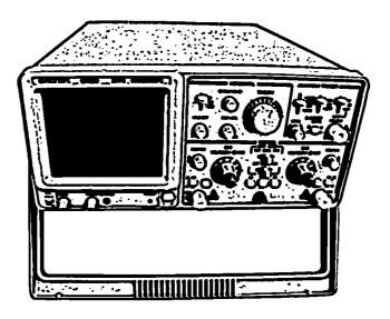
The device shown above is known as an *oscilloscope*, and the screen on the left shows a visual image of a signal or sound wave sent into its input. Eshaal is using it to view the sound waves generated by a microphone placed underneath a tank of fish.
